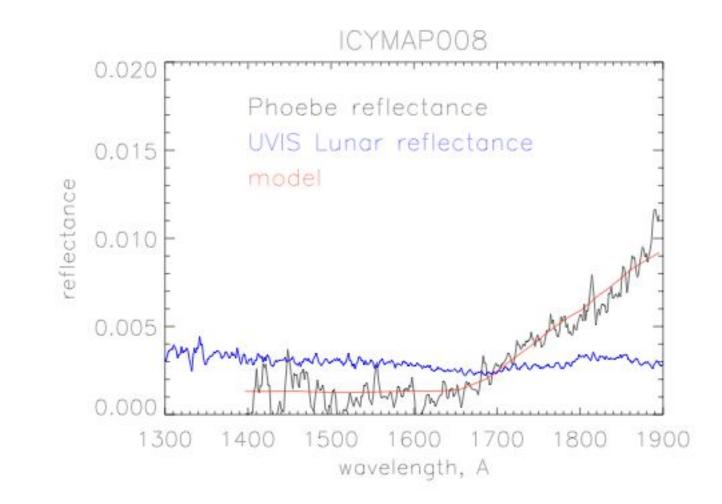
$H_2O$  frost (2 different grain sizes) contributes to Phoebe's FUV spectrum; other (dark) material is similar to carbonaceous chondrite
