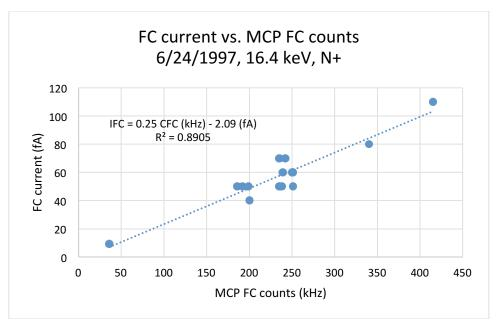
Figure 10. Plot showing the cross-calibration of FC current vs. MCP FC counting rate.
