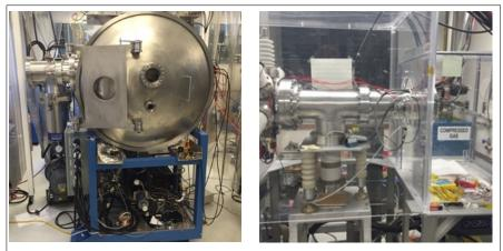
Figure 3. SIMS Facility located at GSFC in bldg. 21, left panel shows rear door of vacuum chamber which contains scan platform and ion beam monitor Quantar imaging microchannel plate system. Right panel shows ion source region of SIMS which can presently be floated up to 15 KV.
