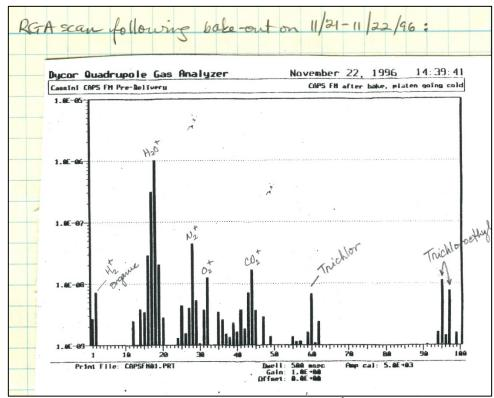
Figure 15a. RGA scan of vacuum chamber residual gases at 1.4 x 10<sup>-6</sup> Torr. The figure was taken from the IMS calibration log book.
