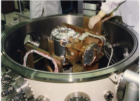
Figure 14. The Flight Model CAPS being mounted in the IBCS for final calibration.
