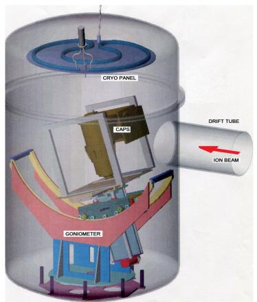
Figure 13. 3-D schematic of the main chamber showing CAPS mounted on the 4-axis motion table. The cryo panel is located at the top of the chamber.
