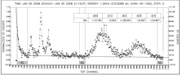
Figure 9. Example of a background fit for a relatively low-count spectrum from the T40 Titan encounter, in which "background-only" intervals can be selected for fitting.
