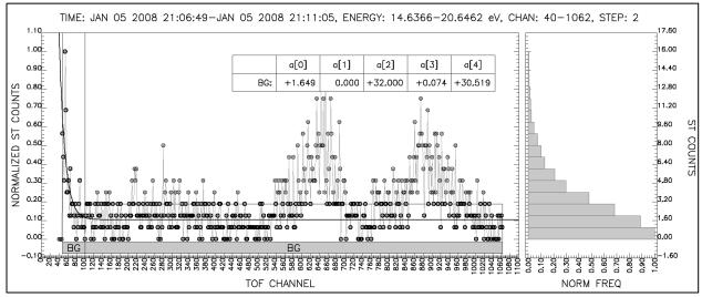
Figure 10. Example of a background fit for a very low-count spectrum from the T40 Titan encounter, in which a histogram of the number of counts greater than or equal to the lower edge of each bar is used to select a subset of points for background fitting.
