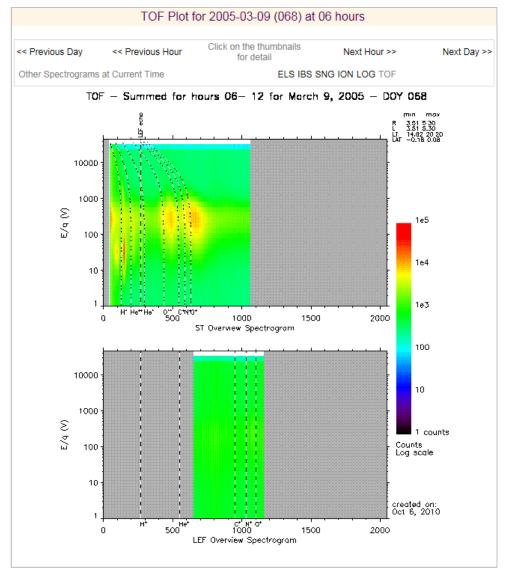
Figure 3. Example of low signal-to-noise ST (top) and LEF (bottom) spectrograms showing total counts summed over a 6-hour period as a function of energy-per-charge and TOF channel.
