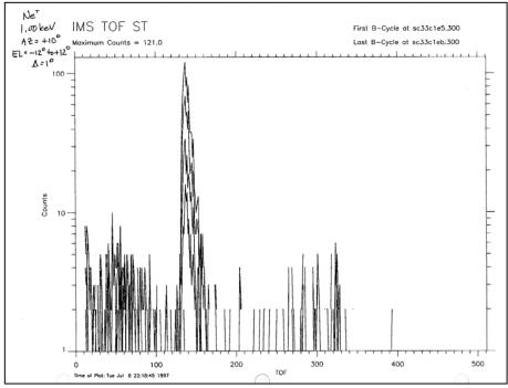
Figure 16. An overlay of ST spectra taken every 2° in azimuth from -12° to +12°.
