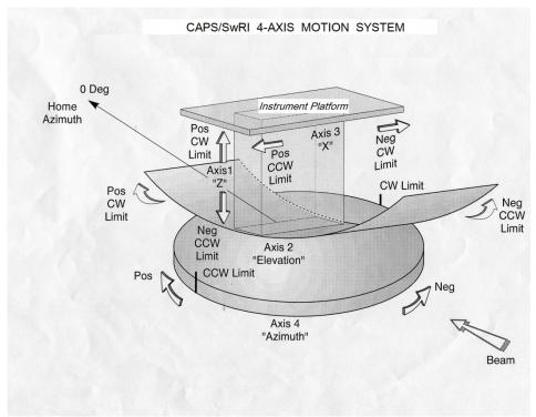
Figure 12. 3-D schematic of the 4-axis motion system. Ion beam enters from lower right.
