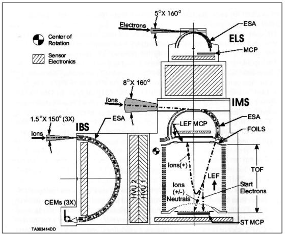
Figure 1. CAPS sensors cutaway with the fields-of-view shown in the azimuthal plane. Characteristic particle trajectories are shown schematically in the LEF region of the IMS.
