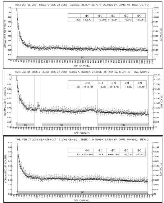
Figure 8. Characterization of background model using summed ST spectra. The model fits are indicated by solid black lines and fit parameters are tabulated in the insets. Filled gray circles represent the summed raw data and open black circles represent the pattern-corrected data.
