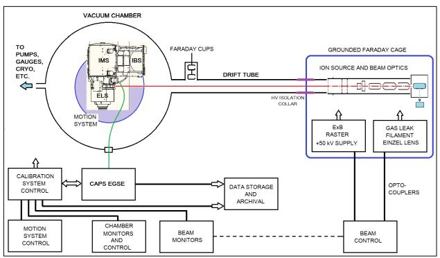
Figure 7. Schematic of the Ion Beam Calibration System (IBCS).
