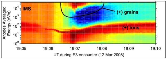
Figure 4. Example of a complex SNG spectrum illustrating strong variation in IMS background levels within the duration of a single TOF integration period (i.e. B-cycle). This highlights the importance of selecting background levels on a B-cycle by B-cycle basis. The figure is taken from Hill et al., 2012.
