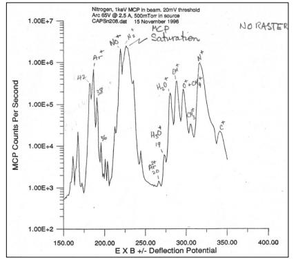
Figure 11a. Mass spectrum of ion beam taken with the MCP Faraday cup with no raster. The figure was taken from the IMS calibration log book.
