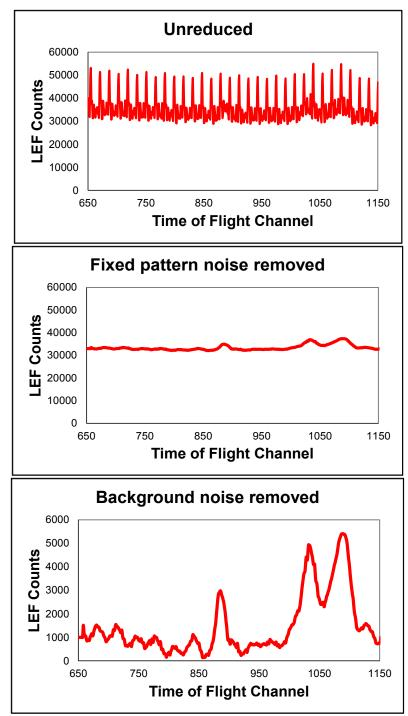
Figure 5. Raw LEF spectrum (DOY 68, 2005). LEF ion counts vs. TOF channel shown with background and repeating pattern noise (top), with repeating pattern noise reduced (middle), and with repeating pattern noise reduced and background subtracted (bottom).
