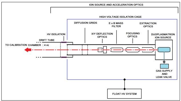
Figure 9. Schematic of the ion source and beam acceleration optics.
