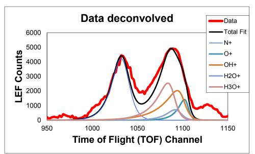
Figure 13. Best-fit sum of LPP peaks for the LEF data corresponding to the ST data in Figure 5.
