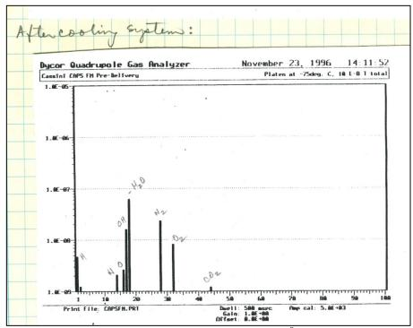
Figure 15b. RGA scan of vacuum chamber residual gases at 9.0 x 10<sup>-8</sup> Torr. The figure was taken from the IMS calibration log book.
