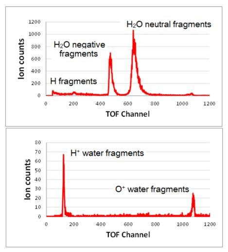
Figure 11. 500 eV ST water ion spectrum (top) and 500 eV LEF water ion spectrum (bottom) from postlaunch calibration measurements.
