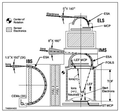
Figure 6. Cutaway schematic of the ELS, IBS and IMS optics showing their component relationships, orientations, optics, and fields-of-view (FOV).
