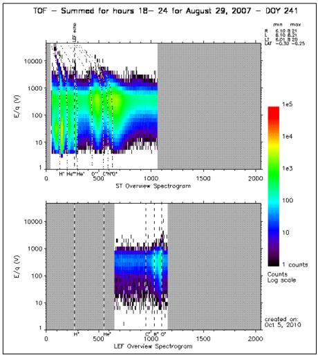
Figure 2. Example of high signal-to-noise IMS ST (top) and LEF (bottom) spectrograms showing total counts summed over a six-hour period as a function of energy-per-charge (Y-axis) and TOF channel (X-axis).
