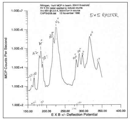
Figure11b. Mass spectrum of ion beam taken with the MCP Faraday cup with maximum raster. The figure was taken from the IMS calibration log book.
