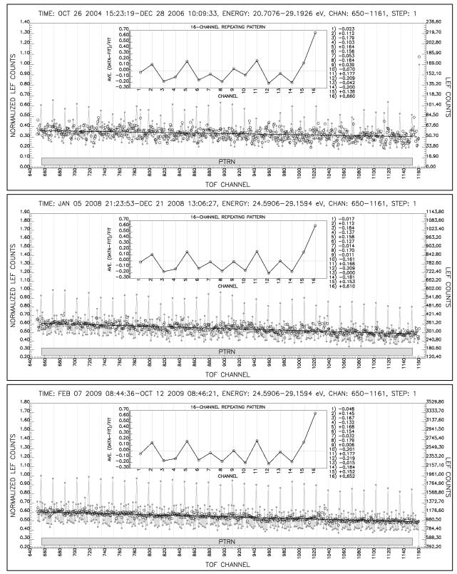
Figure 6. Characterization of RPN using summed LEF spectra. The 16-channel patterns extracted from the spectra are shown in the insets. Filled gray circles represent the summed raw data and open black circles represent the pattern-corrected data.
