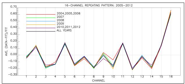
Figure 7. The repeating pattern extracted from LEF spectra summed over six different periods between 2004 and 2012, as seen in the legend. The pattern is expressed as a relative difference between the data and a linear fit to the data. Variation in the pattern is shown to be minimal over the duration of the mission.
