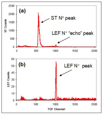
Figure 15. ST and LEF spectra for N<sup>+</sup> taken from calibration data.
