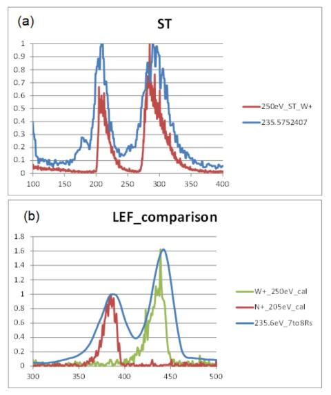
Figure 14. Comparison of 250 eV ST calibration peak widths (a) and comparison of 250 eV LEF calibration peak widths (b) to those observed in flight. Flight data is represented by a blue line in each plot, and calibration data is represented by red and green lines.
