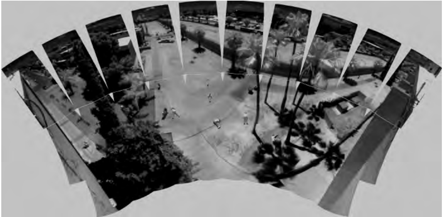
Figure 5.8-4 - A mosaic of 30 DISR images taken from the roof of the Kuiper building (~13 m high), in conformal conic projection showing the U of A mall area.
