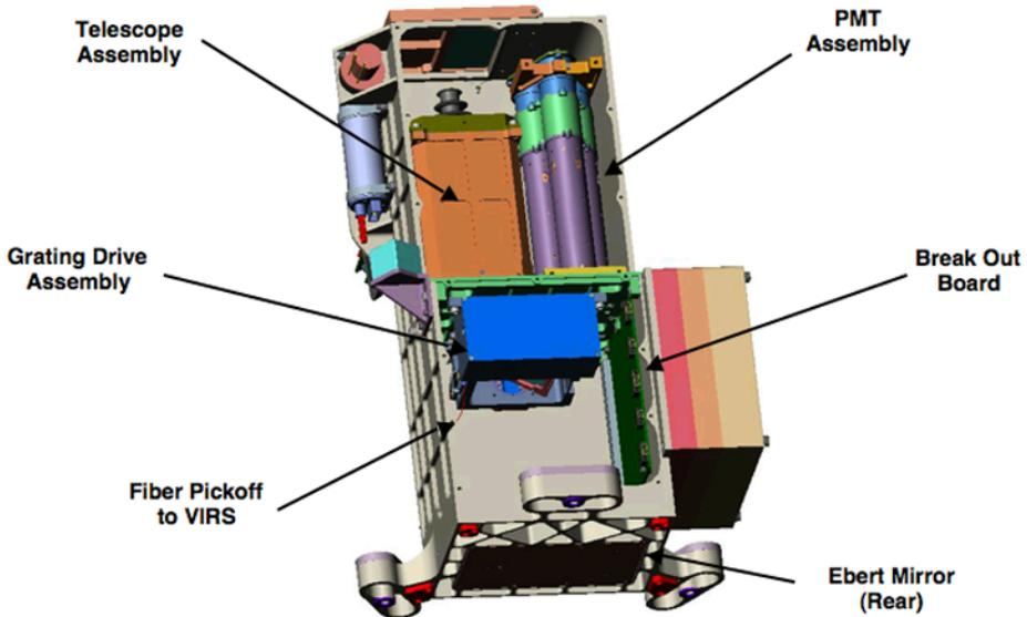
**Fig. 10** Solid-model drawing showing the UVVS components
