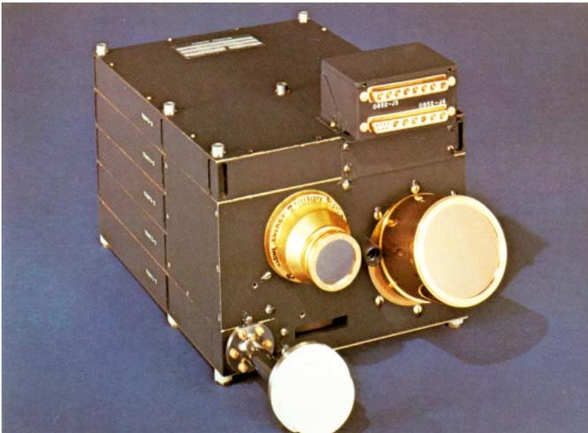
Figure 4-5. Charged particle detectors were used to study the life history of cosmic rays in the Solar System and to study radiation trapped in the Jovian and Saturnian magnetospheres.
