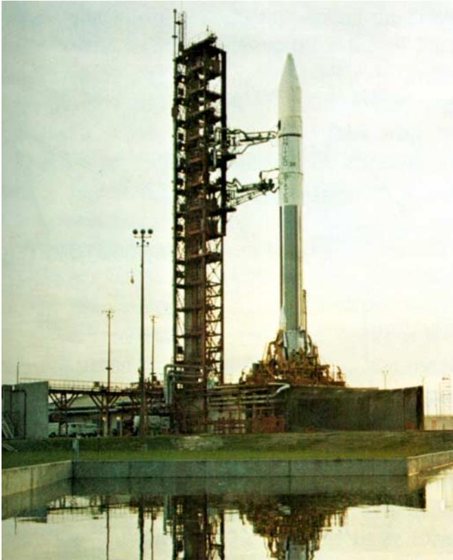
Figure 2-1. Missions to the giant planets required that the spacecraft reach the highest launch velocity yet achieved by any man made object, over 51,500 km/hr (32,000 mph). An Atlas-Centaur launch vehicle was used, equipped with a third upper stage.
