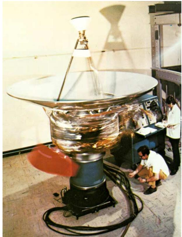
Figure 3-2. Each *Pioneer* spacecraft was stabilized by rotation, as shown in this photograph of a spacecraft under spin test.
