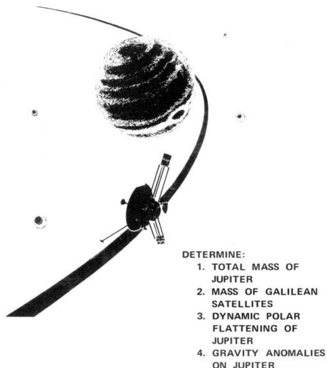
Figure 4-13. A celestial mechanics experiment determined the masses of Jupiter and its Galilean satellites (Io, Europa, Ganymede, and Callisto); of Saturn and its largest satellite, Titan; and of Saturn’s rings. Also, previous findings about the polar flattening of Jupiter and Saturn were verified. This diagram shows the experiment for Jupiter.
